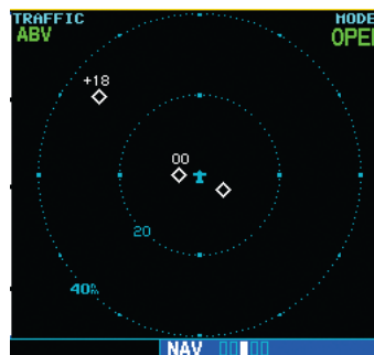
Traffic Page showing Bendix/King KTA 870/KMH traffic near the 40 nautical mile range, at 10 o'clock above.
