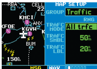
Selections for configuring traffic data are made from the Map Setup Menu on the Map Page.
