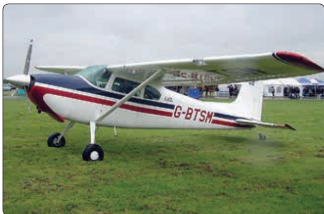
Figure 7-38. Tailwheel landing gear.
