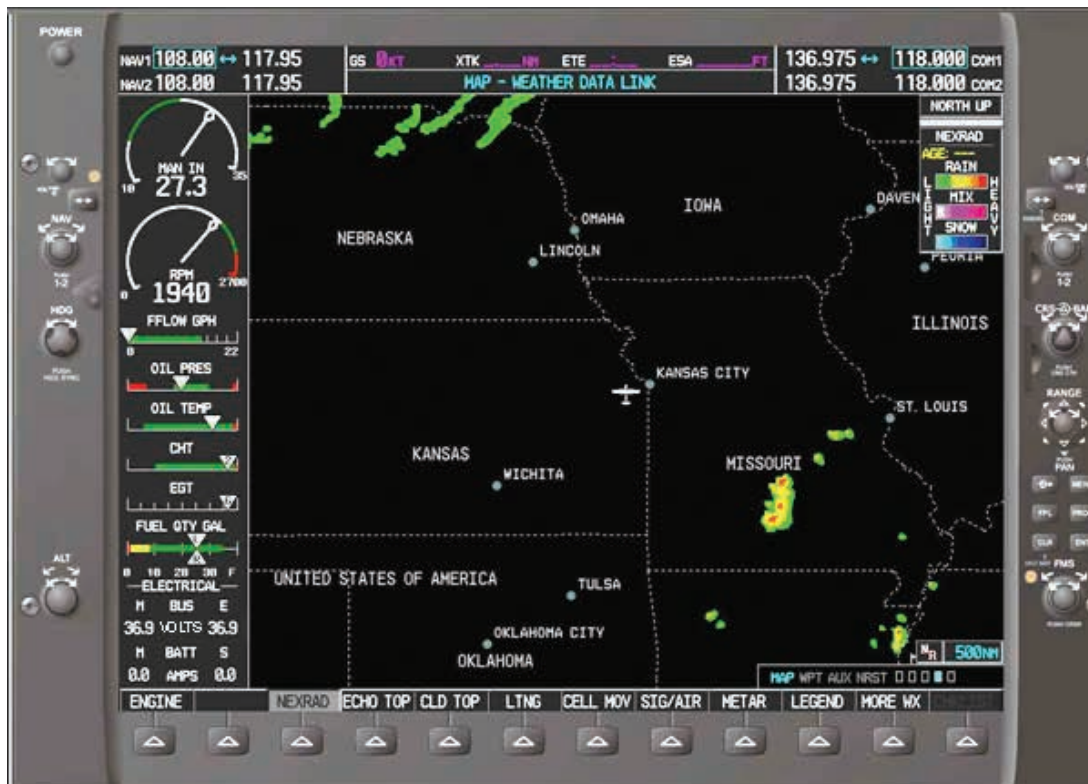
Figure 13-18. NEXRAD radar display (500 mile range). The individual color gradients can be easily discerned and interpreted via the legend in the upper right corner of the screen. Additional information can be gained by pressing the LEGEND soft key, which displays the legend page.
