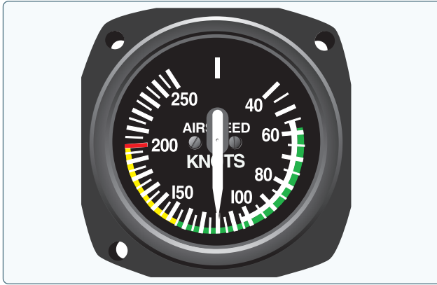
Figure 9-1. Single-engine airspeed indicator.
