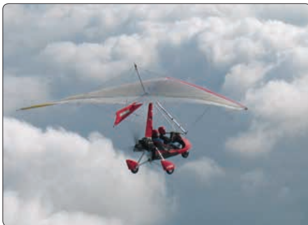
Figure 5-19. A weight-shift control aircraft.
