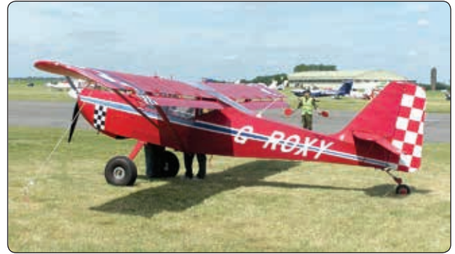
Figure 6-9. Flaperons on a Skystar Kitfox MK 7.
