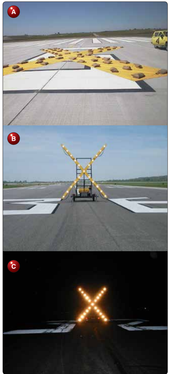
Figure 14-27. (A) Yellow “X” placed on surface of temporarily closed runways. (B) Lighted “X” placed on temporarily closed runways. (C) Lighted “X” at night showing a temporarily closed runway.
