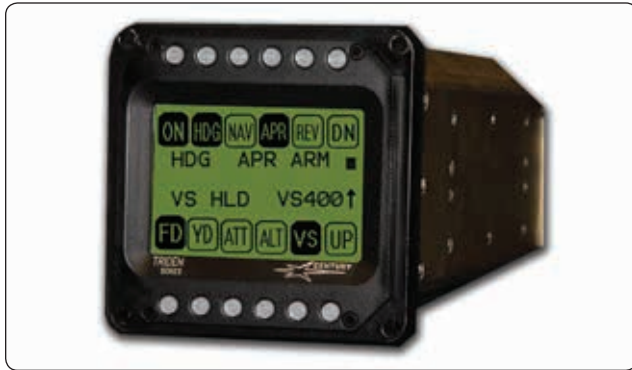
Figure 2-23. An example of an autopilot system.
