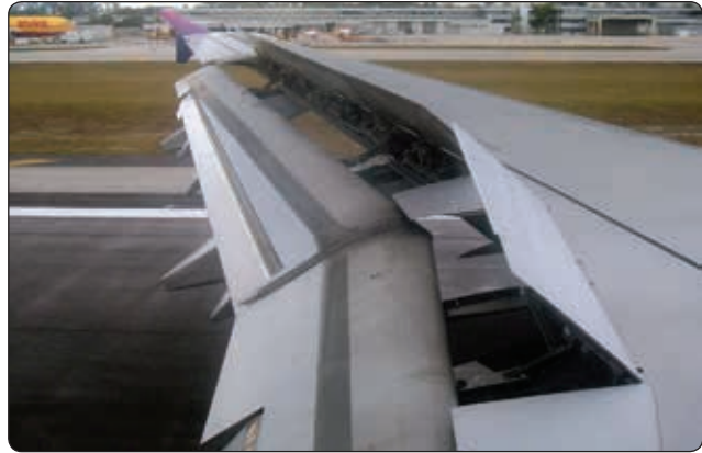
Figure 6-19. Spoilers reduce lift and increase drag during descent and landing.
